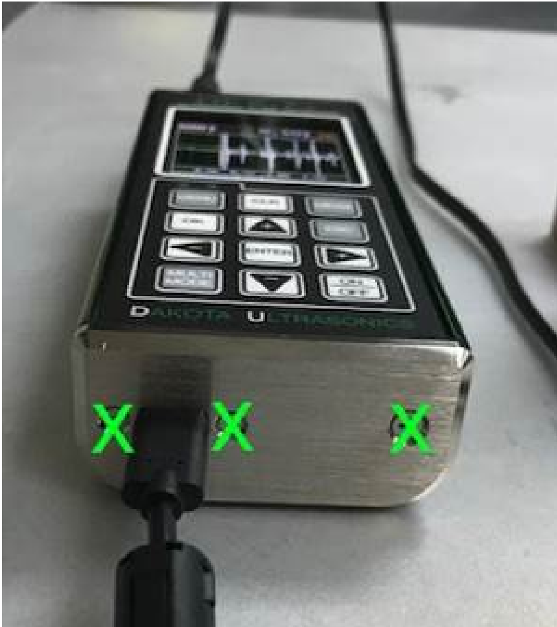
Photograph 8. ESD Test Points – Bottom of EUT
