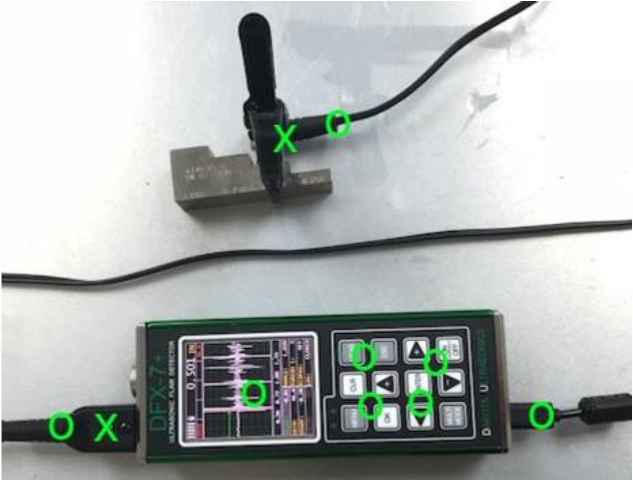
Photograph 7. ESD Test Points – Front of EUT
